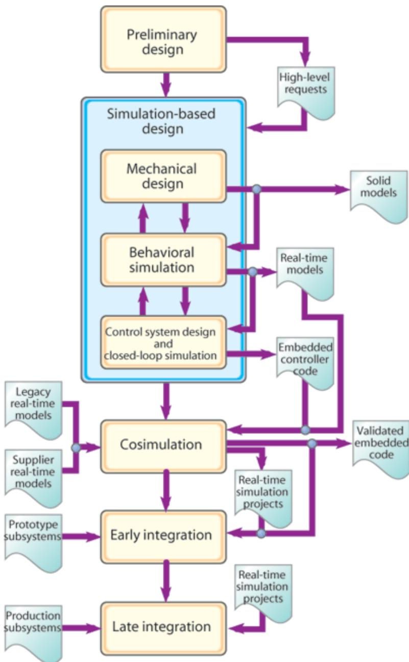
**Figure 1: The simulation-centric process flow**
