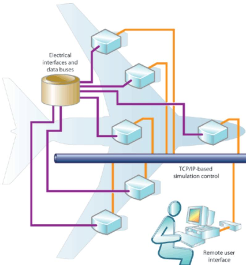
**Figure 3: Moving subsystem models and embedded system code to cosimulation**
