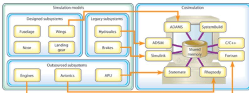
**Figure 2: Moving subsystem models and embedded system code to cosimulation**
